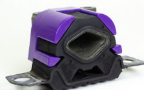
Figure 3: Fit insert into mount
