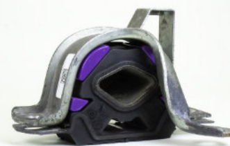
Figure 4: Refit top half of mount
