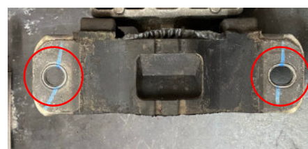
Figure 1: Swaged bolt holes to be drilled
